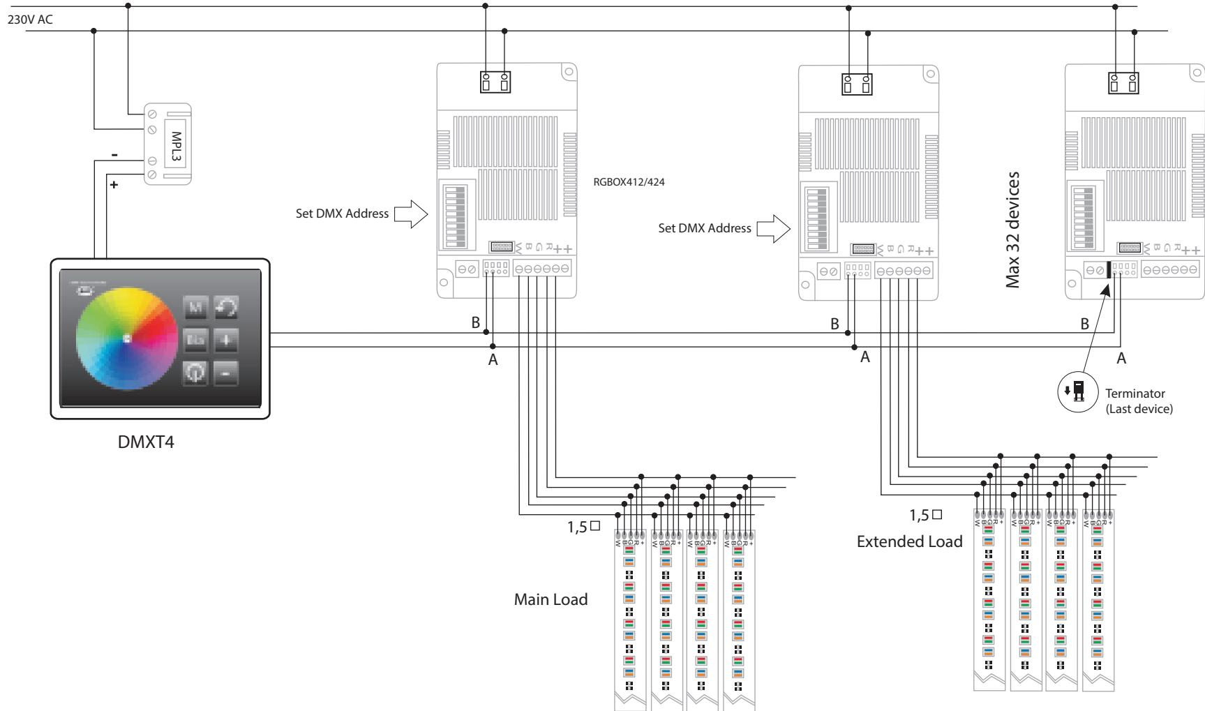
RGBOX4 + RGBA or RGBW DMX controlled system with extension (optional)
