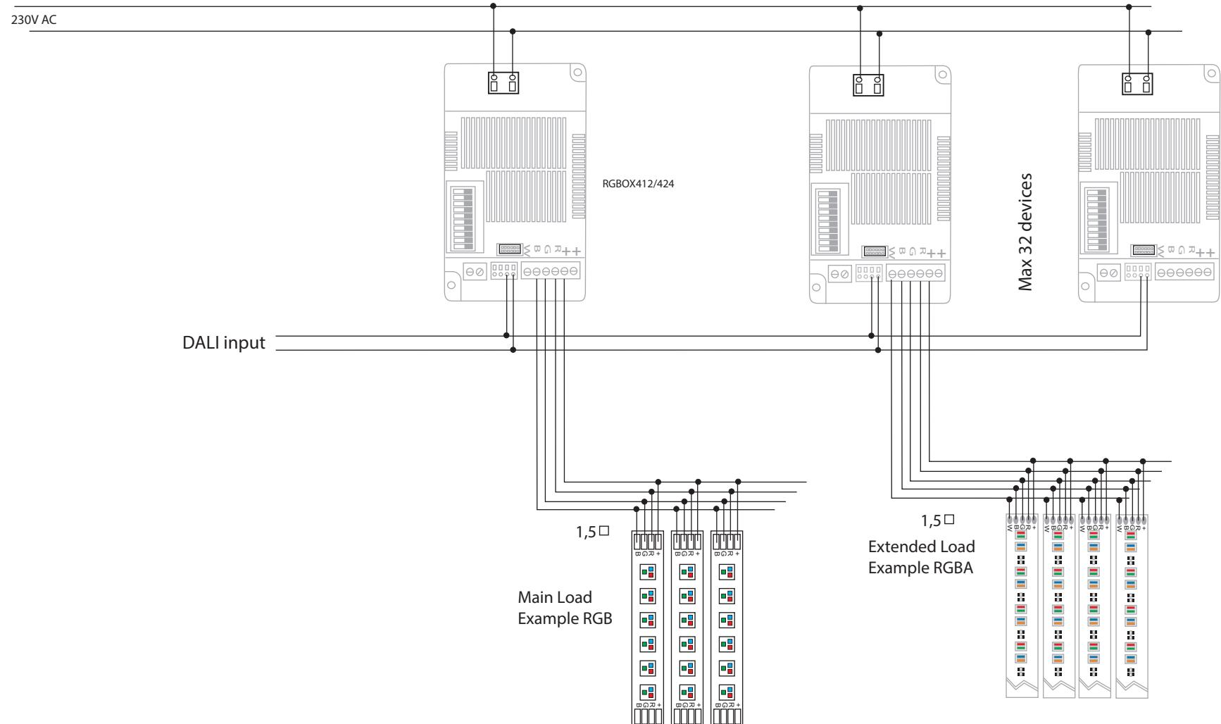
RGBOX4 + RGB or RGBA DALI controlled system with extension ( optional)
